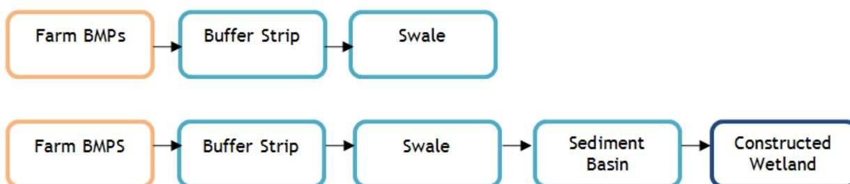
Figure 2 - Possible locations of vegetated swales and drains in farm run-off treatment trains.
