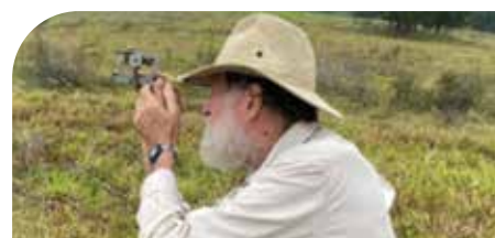
Tools of the trade – Darryl using a Abney Level (Hand Level) to measure slope.
