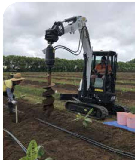
An excavator was used to auger a narrow hole for the lysimeter to a depth of 2.1 metres, in 20 cm increments. The soil was placed into labelled tubs for re-packing the hole.
