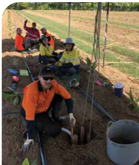
After the lysimeter was placed into the ground teams of workers manually replaced and packed the soil with wooden rods to replicate the undisturbed soil conditions.
