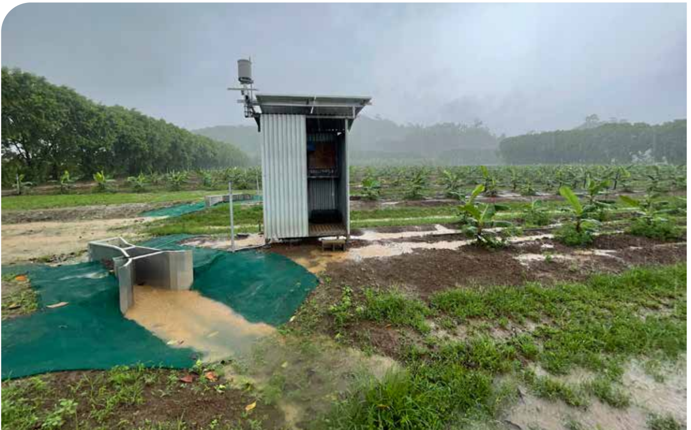
Surface water running through the flumes after cyclone Jasper (mid-December 2023). Samples are collected from this flume and stored in a refrigerated state in the monitoring shed until collection.
