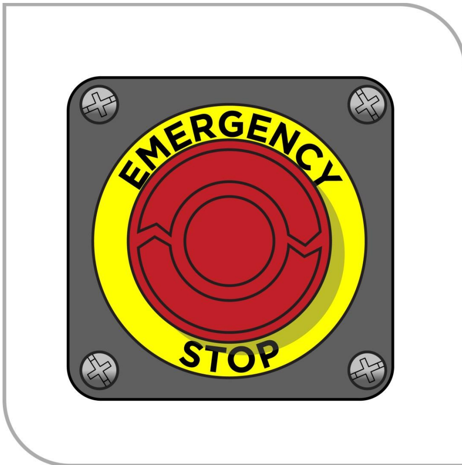
Figure 8 Emergency stop button
