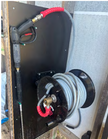
The system delivers high pressure through a long hose, ensuring sufficient reach to the wash-down and disinfecting pad.
