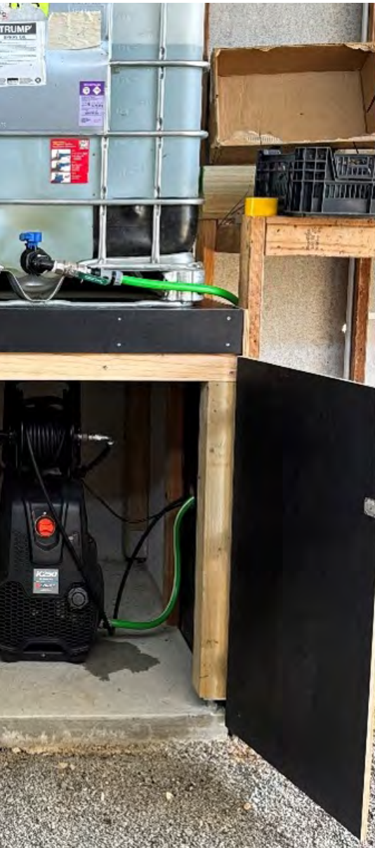
The system delivers high pressure through a long hose, ensuring sufficient reach to the wash-down and disinfecting pad.
